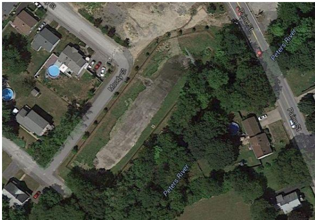
Figure 20 Detention pond adjacent to Peters River at Paine St.
