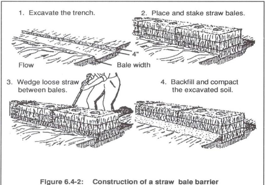
Installation of hay-bales for sediment retention purposes
