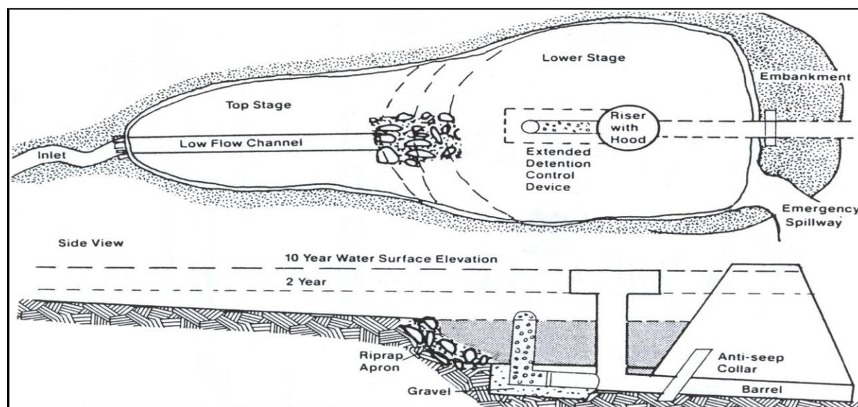
Schematic design of a dry extended detention pond
